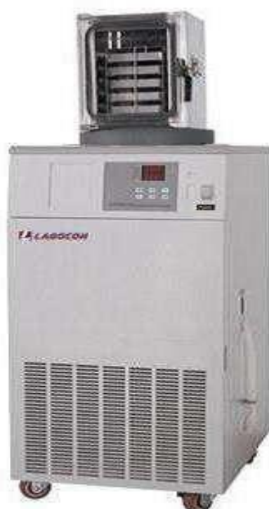
Acrylic Drying Chamber with 3 Shelves
