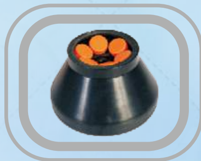
Angle Rotor AR-5: 6x50 ml
