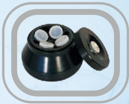
Angle Rotor AR-7: 4x100 ml
