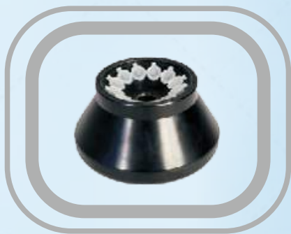
Angle Rotor AR-3: 12x10 ml
