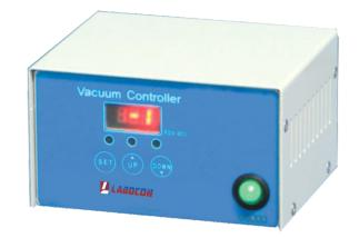
Solid state module maintains precise control ( $\pm$ 3%) of the system vacuum by cycling the pump on/off as required.
